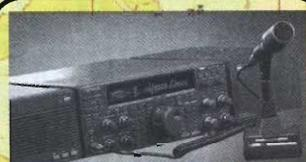
**TS-850 S/AT** - Ricetrasmittitore HF per SSB-CW-AM-FM-FSK - 100 watt out
